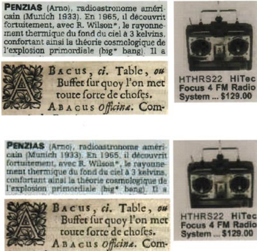
Fig. 5. Comparison of DJVU at 300 dpi (top three pictures) and JPEG at 100 dpi (bottom). The pictures are cut from encyc2347.tif (top), pharm1.tif (bottom), and hobby002.tif (right). The file sizes are given in Table II. The two methods give files of similar sizes, but very different qualities.
